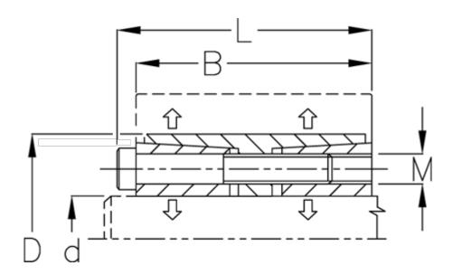
$\begin{array}{lll} \text{B mm} & = 102 \\ \text{d H8 mm} & = 100 \\ \text{D mm} & = 145 \\ \text{Fit tolerance} & = \text{Aksel h8, Nav H8} \\ \text{F kN torque} & = 289.0 \\ \text{L mm} & = 114 \\ \text{M mm} & = \text{M12} \\ \text{P N/mm2 surface pressure on shaft/hub} = 36 \end{array}$
